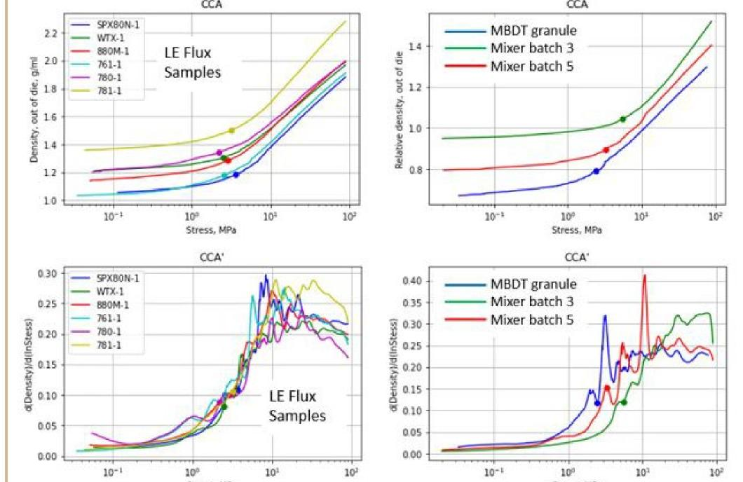
Compaction results from the DOE and LE flux samples were compiled into a statistical model, predicting yield stress as a function of material and process parameters. In addition to effects of raw powder milling and pre-wetting, the silicate binder had a strong correlation with calcining schedule, suggesting the importance of calcining following granulation.
