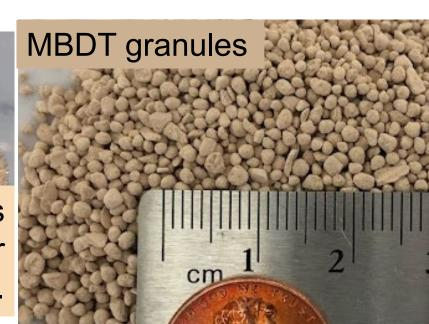
As a variant of DPT, a moving-bed drop-templated process (MBDT) was developed, using a food processor to create a moving bed of powder with a pulse of impinging droplets provided by a syringe pump.
