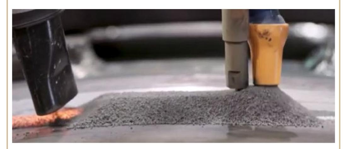
Lincoln Electric (LE) is considering upgrading the granulation process used to produce SAW flux, with a goal of improving process yield, granule structure, and facilitating changes between fluxes in use.
